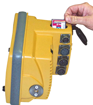
The Topcon 9168 control box, above, displays detailed elevation data for the jobsite. This data is imported via a compact flash card, shown being inserted, below, into the top of the control box.
