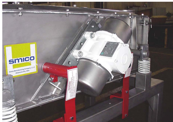
Custom dimensions in a SMICO MVC 495F vibrating screen allowed General Materials to replace a plant's screen, wash and rinse operations with little alteration to an existing plant.
