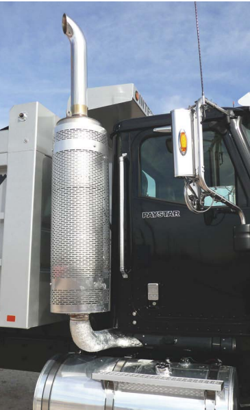
The diesel particulate filter doubles as a muffler, but its bulk pushes the body back almost 2 feet and extends the truck's overall length. There are other ways to mount the DPF, though.
